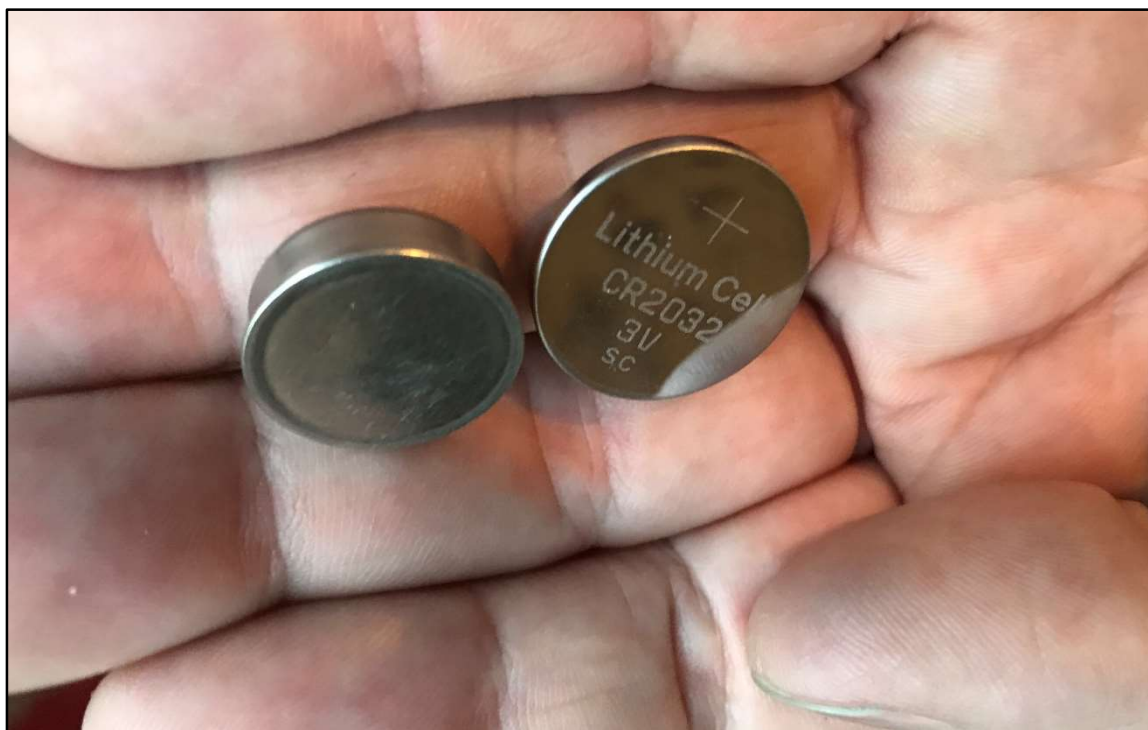
Figure A4.1. Standard thermo button compared to a CR2032 Litium battery.
